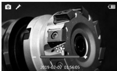
Figure 5-6 Adjusting LED Brightness, example screen
