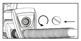
3. Replace the battery cap carefully and do not over tighten
