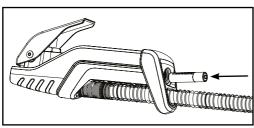
2. Slide the batteries into the inflator with the positive end facing out of the inflator
